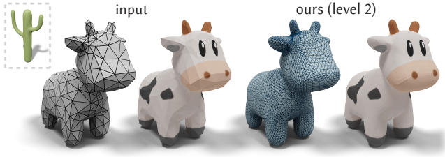
Fig. 3. Neural subdivision can adapt to different input triangulations and output a high-resolution surface mesh accordingly. This enables us to use it directly in the graphics pipeline such as texture mapping.
