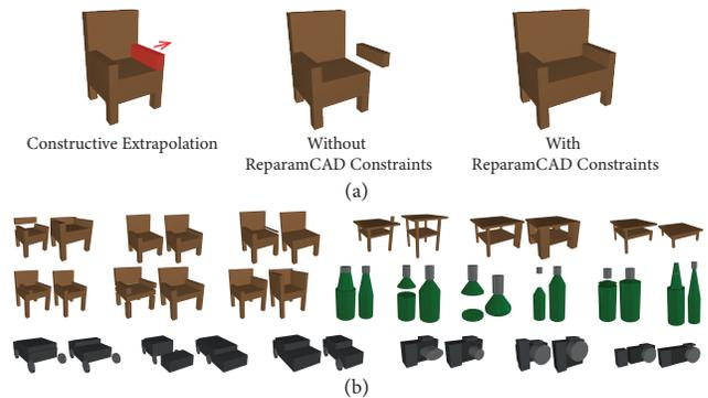
**Figure 4: (a) Applying an extrapolative edit to a model can lead to broken geometry, but the constraints we discover prevent this and result in meaningful global edits from local changes. (b) A selection of random extrapolative edits without ReparamCAD (left) and with (right). ReparamCAD maintains geometric coherence.**
