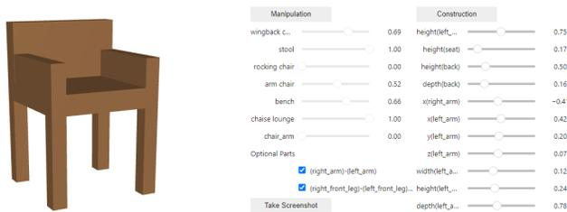
**Figure 3: ReparamCAD’s user interface.** Users are presented with two complimentary views of the constrained reparameterization space. The sliders on the left interpolate between discovered variations as a weighted average, while those on the right control the free variables after reparameterization. Checkboxes allow toggling of discrete sets of removable parts.
