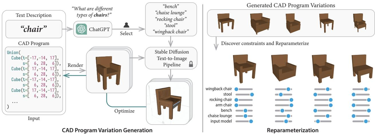
**Figure 1: ReparamCAD takes a parametric 3D model and a corresponding text description as input and generates a re-parameterized version of the model as output. It uses ChatGPT and user guidance to generate text prompts describing variations of the input model and uses stable diffusion to optimize the CAD parameters towards these prompts. The resulting variations are used by the constraint discovery system to identify common constraints across all designs.**
