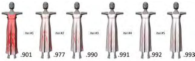
Figure 4: Pattern adjustment following the hem elongation in Figure 6. Left to right: iterations zero to 5. Color (red to white) shows intrinsic triangle stretch w.r.t. to corresponding target geometry (scale from 0.8 to 1 with 1 being optimal). The number next to each garment is the average stretch.
