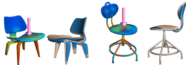
(a) Wood: \rho = 900 \text{ kg/m}^3 , E = 12.6 \text{ GPa} , \nu = 0.45 (b) Metal: \rho = 8050 \text{ kg/m}^3 , E = 200 \text{ GPa} , \nu = 0.3
