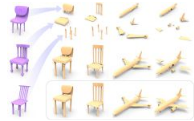
Figure 1: Our deep learning framework, COALESCE , assembles 3D shapes by a learning-based approach to synthesize part connections. Given a set of unaligned, roughly cut parts with possibly mismatched joint regions (top row: all parts come from different shapes), the alignment module of our network can learn to arrange these parts into a plausible configuration (middle row). However, this still leaves gaps and geometric/topological mismatches at the joints. After eroding the input parts in advance, our joint synthesis module creates connecting regions, which are stitched to the input to create seamless assemblies (bottom row).
