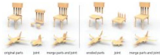
Figure 6: Comparison of two networks that synthesize part connections from original parts before erosion (left) and from eroded parts (right). Incorporating erosion better resolves geometric and topological mismatches.
