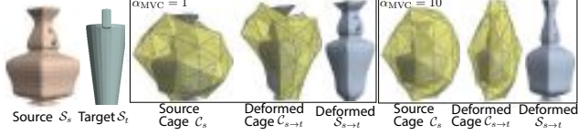
Figure 12: Effect of \mathcal{L}_{MVC} . Higher regularization yields more conservative deformations.
