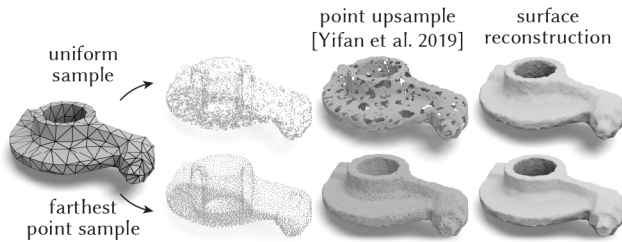
Fig. 5. One can use existing point upsampling methods to refine coarse meshes by (1) sampling, (2) upsampling [Wang et al. 2019b], and (3) reconstruction [Kazhdan and Hoppe 2013]. However, this may lead to artifacts since it lacks information about the surface, and requires the use of expensive surface reconstruction as a post-process.
