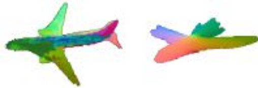
Fig. 4: Visualization of learned surface parameterization with a (left) Chamfer loss and (right) gnomonic mapping loss. Discontinuities in colors indicate self-intersections.
