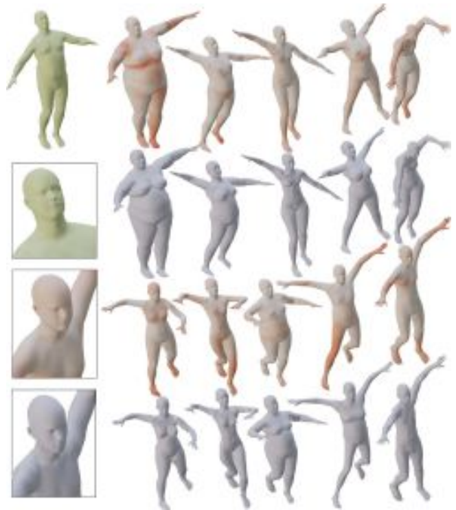
Fig. 10. Learning to morph humans into other humans. We train our network to receive Pointnet [Qi et al. 2017] encodings of two random humans in random poses from the STAR [Osman et al. 2020] dataset, and map one into the other. Source mesh is shown in green, targets in blue and the deformations colored w.r.t. error (reddest being 0.1). The network correctly maps the humans, and in places where the pointnet encoding is not descriptive (e.g., the faces), defaults to an accurate detail-preserving deformation of the source.
