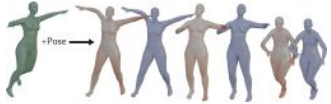
Fig. 6. Learning to re-pose humans. We learn the STAR [Osman et al. 2020] dataset’s pose parameter space: the network is given a mesh of an arbitrary human (left, green) in an arbitrary pose, along with the parameters of the pose it should be moved to, and re-poses it correctly. Ground truth colored in blue, and predictions w.r.t. error (reddest being 0.05).
