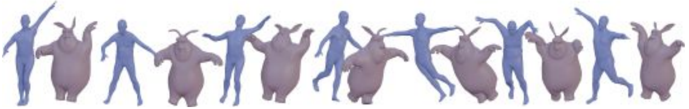
Fig. 7. Generalization of the re-posing network to Big Buck Bunny. Our network was trained solely on training samples of human meshes from the STAR [Osman et al. 2020] dataset, and is applied here to the bunny – an unseen mesh, with different triangulation and geometry. We show a STAR mesh in blue, in the ground-truth pose, and the network’s reposing of the bunny. The training set consists of one fixed triangulation, which is different than that of the bunny, hence this result can only be achieved by a triangulation-agnostic framework.
