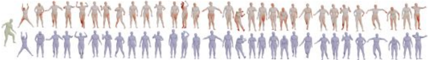
Fig. 8. Learning to register humans. Our network learns to correctly register any input random SMPL [Bogo et al. 2016] model to itself in arbitrary poses. Source in green, targets in blue, and the deformation colored based on error.
