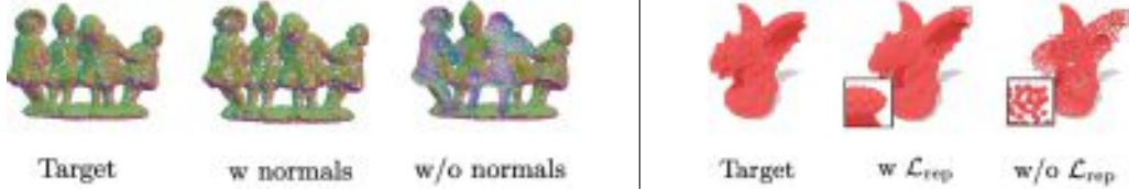
Figure 4: Impact of the normals and the repulsion loss. Note the variation of the color-coded normal directions (left) and the variations in the point density (right).
