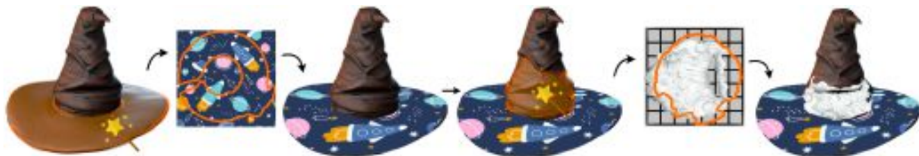
Figure 1. DA Wand enables interactive decaling through a conditional selection of local distortion-aware patches. Our method identifies large patches within both developable and high-curvature regions which induce a low distortion parameterization.
