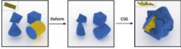
Figure 6. Generation of our “near-developable” synthetic dataset: we draw random geometric primitives, deform them, and apply a CSG union to obtain our final synthetic shape, while transferring the correspondence to the original segmentation (yellow). UVs of the corresponding segmentations are shown in the insets.
