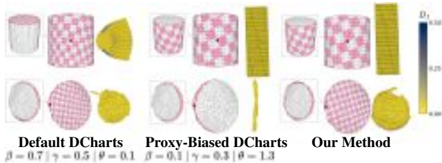
Figure 7. Segmentations predicted by DCharts with default parameters ( Default DCharts ), DCharts biased towards the developability proxy energy ( Proxy-Biased DCharts ), and DA Wand ( Our Method ). The parameter values are given for each DCharts configuration. We show results on a cylinder mesh (top row), and an ashtray mesh from our Thingi10k dataset (bottom row). UV embeddings on the right are colored by isometric distortion D_I .
